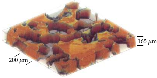
FIGURE 1: Reconstruction of 3D digital cores using confocal laser scanning method (the pore space is opaque (colored) and the solid matrix is translucent). It is obvious that the thickness of 3D digital cores obtained by LSCM method is low. This leads to too little information on the obtained 3D digital core, and the results of numerical simulation using 3D digital cores are not representative. Figure from [43].
