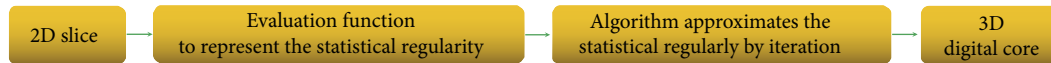
FIGURE 15: Abstraction of the stochastic reconstruction method based on 2D slice statistical constraint features. The effect of 2D slice to 3D digital core is determined by the evaluation function and algorithm. The evaluation function is one of the important parameters that determine the effect of 3D digital core construction.
