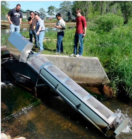
Figure 5. A 400 W pico-hydropower scale Archimedes screw prototype (0.9 m head, 70 L/s design flow) in Canada (Photo credit: Greenbug Energy Inc.).
