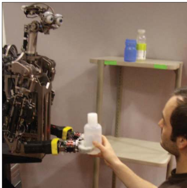
Figure 5. MIT CSAIL robot Domo works with a human to place objects on a shelf [5].
