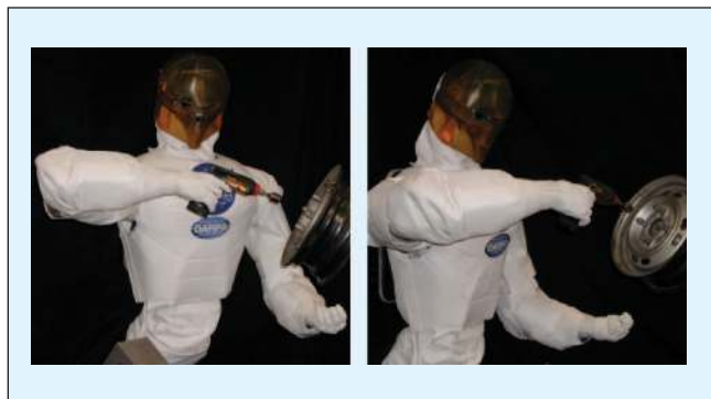
Figure 6. Researchers from Brown and Vanderbilt have been developing methods that enable Robonaut to learn to behave autonomously from teleoperated examples. At the workshop, they presented a method that discovers instances of success and failure from teleoperated examples of Robonaut using a power drill [11].
