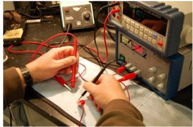
Fig. 4 Four points probe conductivity measurement
