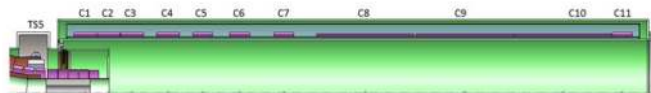
Fig. 2. Layout of the DS coil modules. TS coils are shown on the left.
