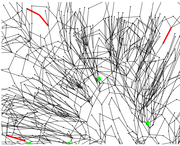
Fig. 3. Failure of the standard OPF shown for a snapshot of the standard OPF solution on Polish grid from MATPOWER [29]; full snapshot is shown in Section III of SI. Color coding and conditions of the experiment are equivalent to these of Fig. 2.
