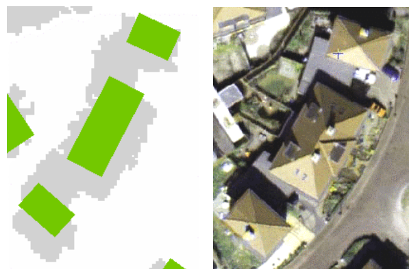
Figure 8: Detected mapping error (see text). Left: laser data segments (grey) and database objects (green (dark)). Right: colour image of a three-line scanner
