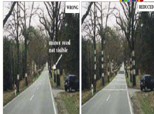
Figure 6: Minor road not visible early enough: unexpected braking and high speed at this point cause rear end collisions [21]
