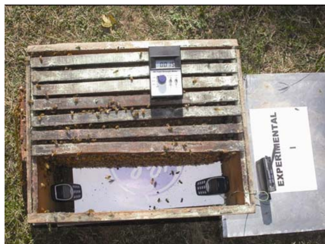
Figure 1. Experimental colony showing placement of mobile phones and power density meter.
