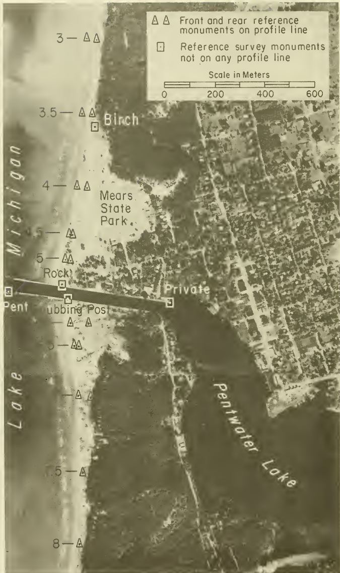
Figure 3. Profile stations in vicinity of Pentwater jetties.
