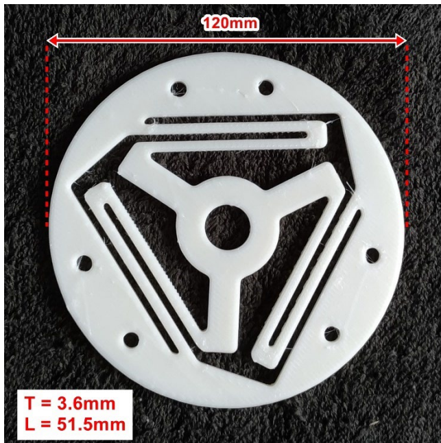
Figure 5. Ortho-planar spring compliant mechanism.
