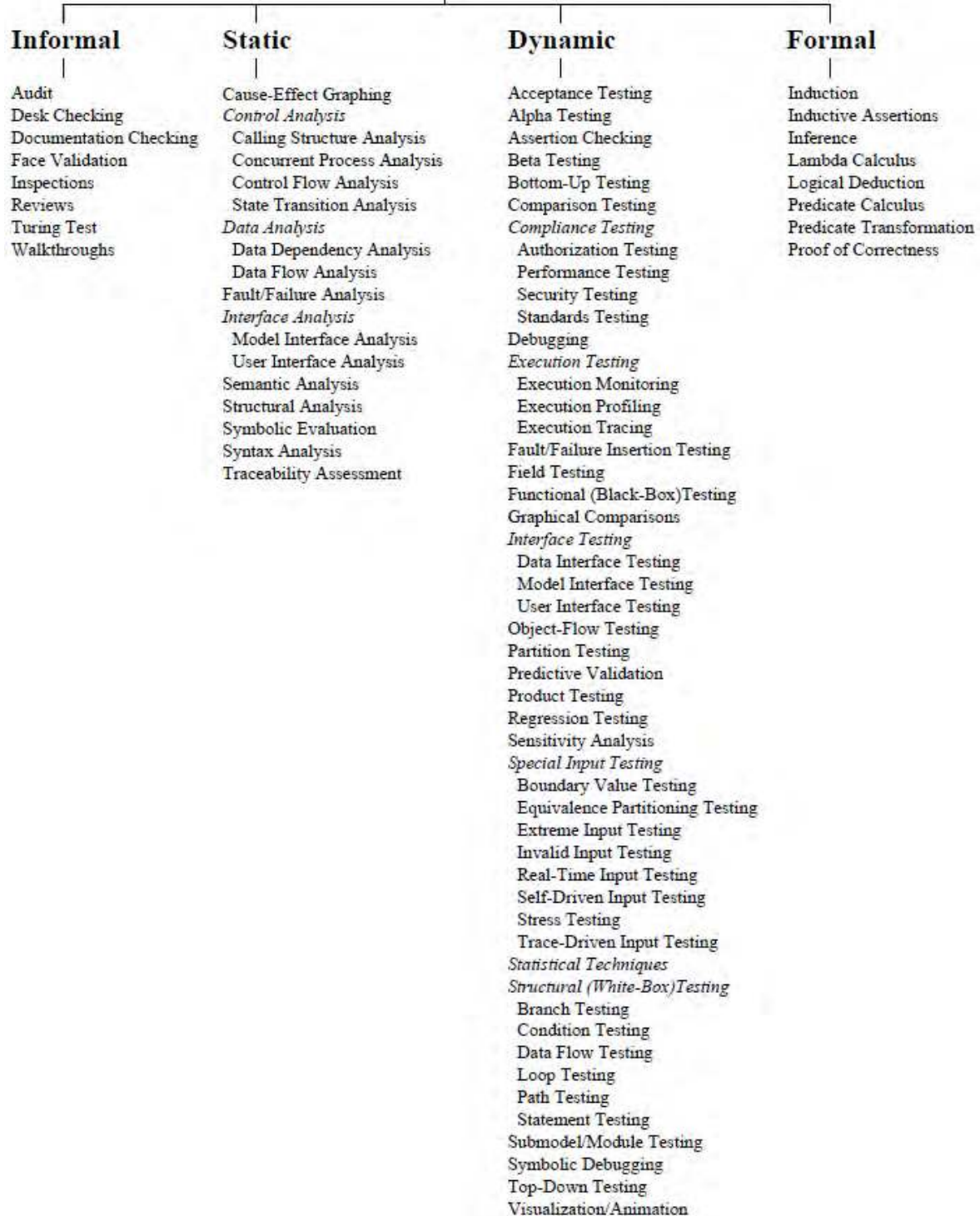
Figure 11. Taxonomy of Verification and Validation Techniques for Conventional Simulation Models (From Balci, 1997)
