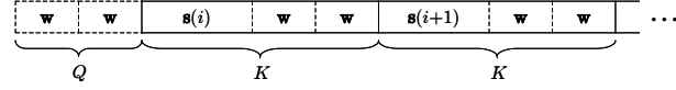
Fig. 2. Example of the UW block structure used to perform deterministic LS channel estimation and tracking.
