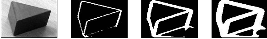
Figure 12.3: Thresholded gradient magnitude with the proposed normalization, using constant threshold and increasing \sigma to the right.
