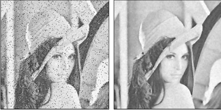
Figure 2.4: An image with Gaussian and salt & pepper noise restored using channel smoothing.
