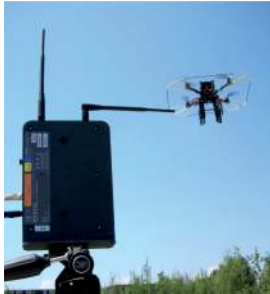
Fig. 2. Orientation of the antennas on the access point
