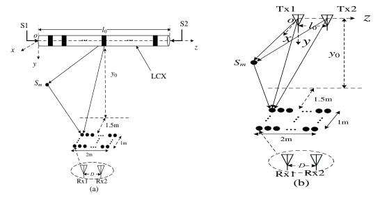
**Figure 13.** MIMO system: (a) transmitting antenna and receiving antenna are LCX and dipole antennas, respectively; (b) transmitting antenna and receiving antenna are both dipole antennas.
