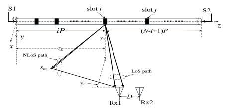
Figure 4. MIMO system with single double-port fed LCX considering both LoS and NLoS paths.
