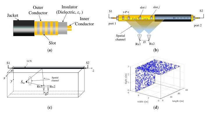
Figure 1. (a) LCX structure for vertical slots; (b) LCX-MIMO system; (c) propagation path of signal for LCX–MIMO system; (d) the distribution of effective scatterer in tunnel, " $\times$ " denotes the scatterer in the side wall or the roof of the tunnel.
