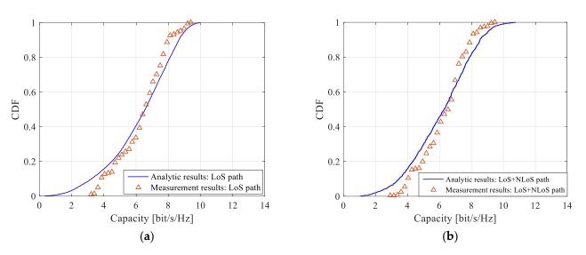
Figure 7. CDF of channel capacity: (a) LoS only path; (b) both LoS and NLoS paths.
