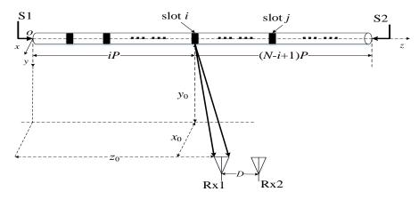
Figure 3. MIMO system with double-port fed of single LCX considering only an LoS path.
