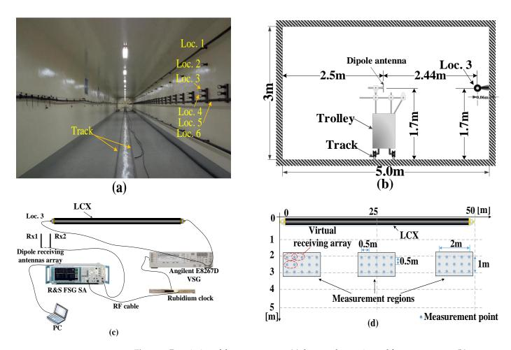
**Figure 5.** Description of the measurement: (**a**) the tunnel scenario used for measurement; (**b**) cross section view of the tunnel; (**c**) connection diagram of LCX MIMO system; (**d**) receiving antenna location.
