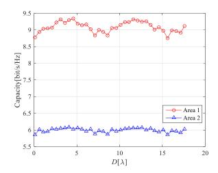
Figure 11. Channel capacity of the LCX-MIMO system for LoS only path.
