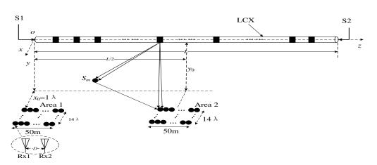
Figure 8. MIMO system with single long double-port fed LCX in tunnel.
