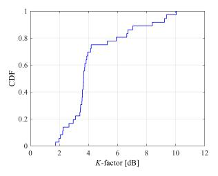
Figure 6. Cumulative distribution function (CDF) of K-factor from LCX MIMO channel measurements.
