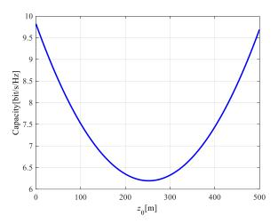
Figure 10. Channel capacity of the LCX-MIMO system with a different location in the tunnel.
