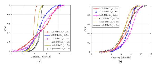
**Figure 14.** Channel capacity for LCX MIMO system and dipole antennas MIMO system: (**a**) LoS only path; (**b**) both LoS and NLoS paths.
