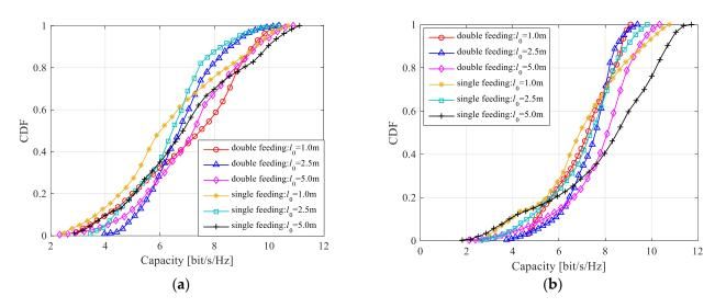
**Figure 12.** Channel capacity of the MIMO system for double-port fed and single-port fed LCX: (**a**) LoS propagation path; (**b**) both LoS and NLoS propagation paths.
