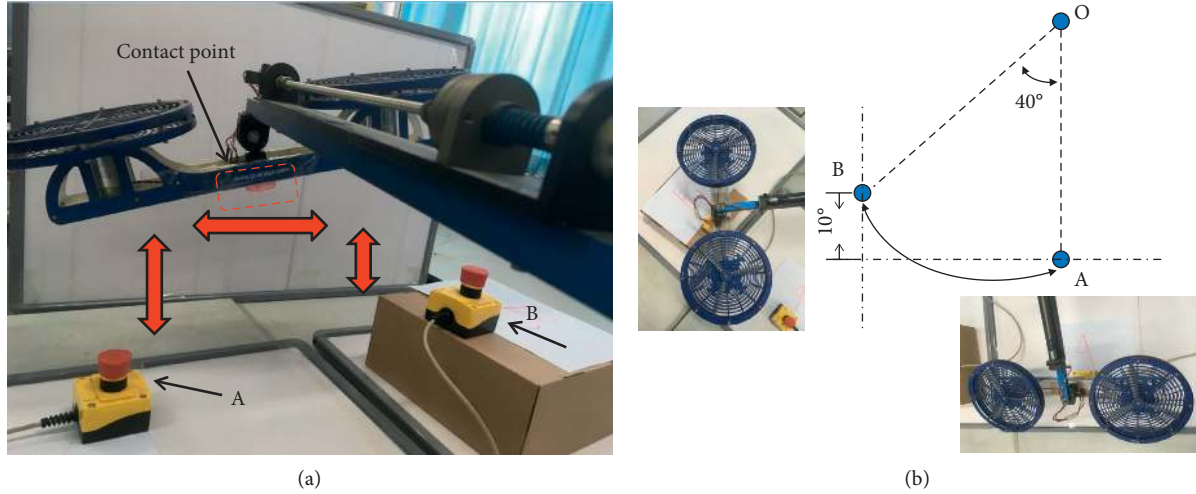
FIGURE 6: The top view of the helicopter flight task. (a) Flight experimental setup; (b) location information and motion curve, the contact point moves from position A to position B and then goes back to position A, and the moving step is 10 degrees in four directions (up, down, left, and right).
