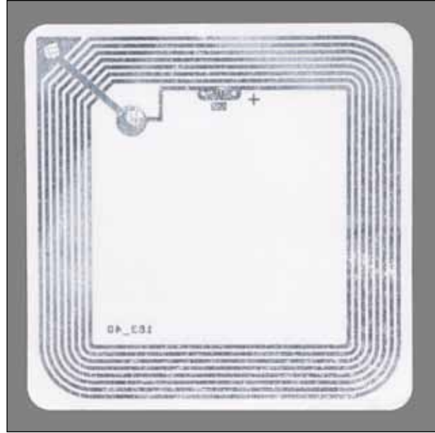
Figure 1.3 RFID Library Solution's square book tag. Image courtesy of RFID Library Solutions. See "RFID Products," RFID Library Solutions website, www.rfidlibrarysolutions.com/#!rfid-products .
