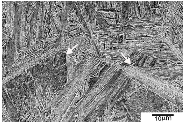
Figure A.10: SEM micrograph shows the structure of sample Sp9c transformed at 300°C for 6 h and strained up to 0.1 strain. Tempering was carried out by heating from 100 to 600°C with \Phi = 10^\circ\text{C min}^{-1} . Arrows point to a bainite sheaf (right) and a tempered-martensite grain (left).
