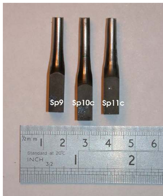
Figure 4.2: Samples corresponding to the tensile curves presented in figure 4.1 fractured in uniaxial tension.
