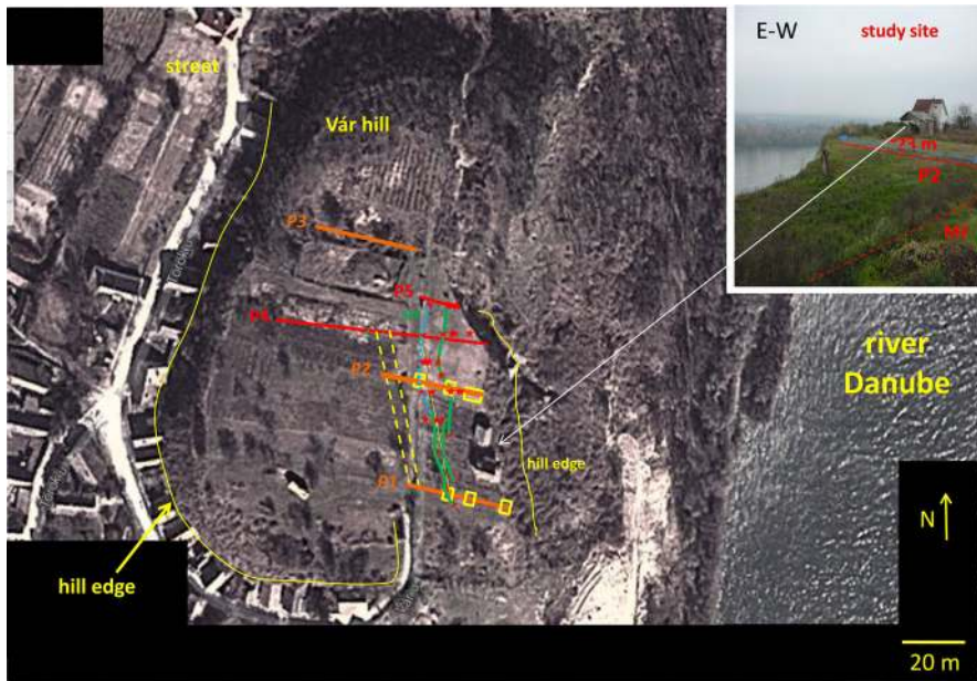
Fig. 2 Google map of the study site. ERT profiles P1, P2 and P3 (brown lines); PreP profiles (red lines P4, P5 and P1). P1 was measured by both methods. The main fracture visible at the time of the measurements (thick dotted blue curve); new fractures developed after the measurements (continuous green curves); the actual scarp (yellow curve); fracture positions (stars); fracture zones in the ERT section (yellow rectangle). Supposed major fractures outside of the active area on the basis of the P1 and P2 PreP profiles (yellow dotted line). (Color figure online)
