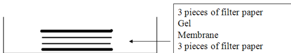
Figure 2.2 Arrangement of gel sandwich
