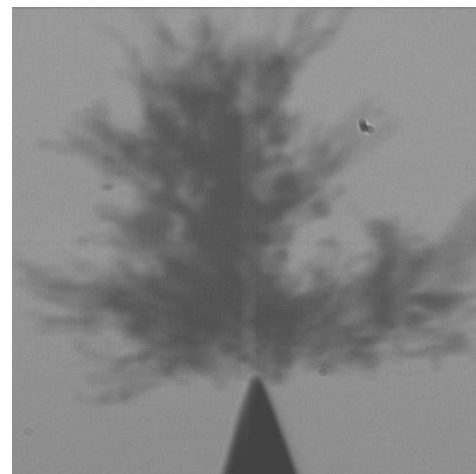
Figure 3 - Typical negative bush like discharge, with apparent charge of 170\text{ pC} recorded at 80.190 \pm 0.198 degrees phase angle.
