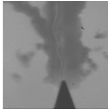
Figure 2 - Typical positive filamentary discharge with visible streamer, apparent charge of 369\text{ pC} recorded at 266.796 \pm 0.198 degrees phase angle.
