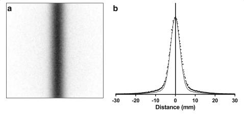
**Fig. 11** Monte Carlo simulated line source image (**a**) and line profile compared to measured (**b**). Simulated assuming 100% density and nominal septal thickness
