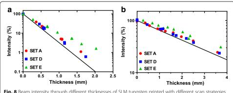
**Fig. 8** Beam intensity through different thicknesses of SLM tungsten printed with different scan strategies and different beam intensities **a** 140 keV, **b** 364 keV compared to the theoretical ideal (solid line)
