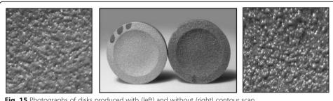
Fig. 15 Photographs of disks produced with (left) and without (right) contour scan
