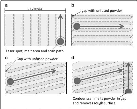
**Fig. 14** Schematic illustration of scan strategies, showing laser spot, melt area, path direction and overlap. **a** Scan path is perpendicular to object face. **b** Scan path is parallel to object face. **c** Scan path is angled from object face. **d** Scan path is angled with the addition of contour scan around periphery of object
