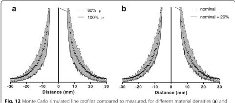
**Fig. 12** Monte Carlo simulated line profiles compared to measured, for different material densities (**a**) and septa thicknesses (**b**)
