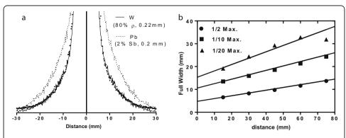
**Fig. 13** Monte Carlo simulated line profiles of tungsten (80%  $\rho$ , 0.22 mm septa) and lead (25Sb, 0.2 mm septa) collimators (**a**) and comparison of measured (points) and simulated (solid line) (tungsten 80%  $\rho$ , 0.22 mm septa) resolution at different distances (**b**)
