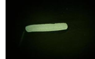
(v) Macro view of formed flat wire electrode size of 2 x 0.6 mm
