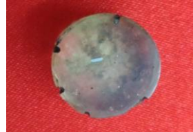
(iii) Macro view of formed flat electrode
