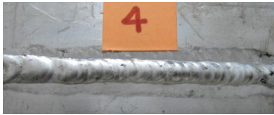
(iii) inclined to the welding direction (expt. trial -4)
