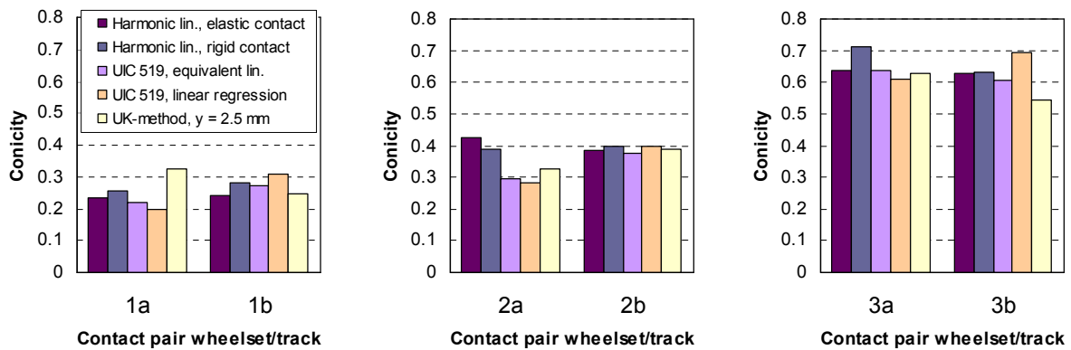
Figure 6. Comparison of the equivalent conicity for the wheelset amplitude of 3 mm of the investigated wheel/rail contact geometry examples.
