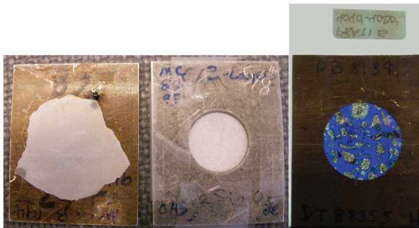
Figure 17. Two methods of mounting samples for (U)SANS analysis. The images on the left shows a sample ground to 150 \mu\text{m} , then floated off the glass slide (originally glued on using super glue) and attached to the Cd mask. The image on the right shows a sample mounted on a quartz glass slide that was then taped directly to the Cd mask. Unlike the samples to the left and middle, the sample on the right consists of drill cutting mounted in epoxy, rather than solid rock, but the method of mounting on quartz glass works similarly well for larger samples (Anovitz, unpb.).
