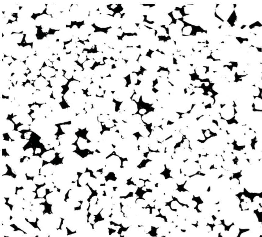
Figure 40. Binary image (pores black, quartz white) of sample 04Wi17b, 100 °C, 8 weeks from Anovitz et al. (2015a). Image is 5.3 mm across.
