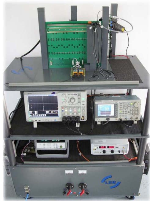
Figure 1. Double pulse measurement test bench with extended features compared to conventional setups.
