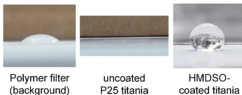
Figure 10. Photographs of water droplets on the filter, on uncoated titania particles on the filter and on HMDSO-coated titania on the filter.
