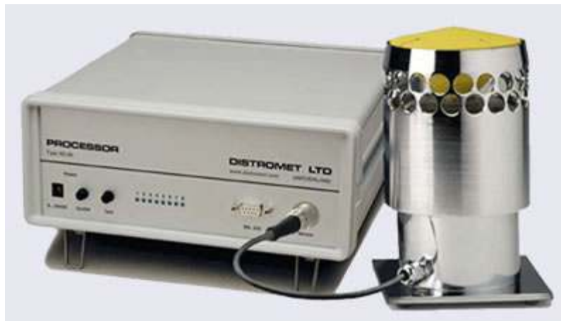
Figure 1.4 Joss-Waldvogel disdrometer based on impact disdrometer principle [5]
