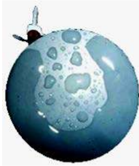
Figure 3.3 Puddle effect: accumulation of water on the hat of the disdrometer
