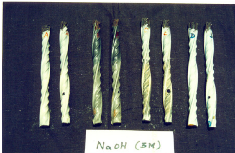
Figure 3. Photograph of coated rebars immersed in 3 M NaOH solution for a duration of 60 days.
