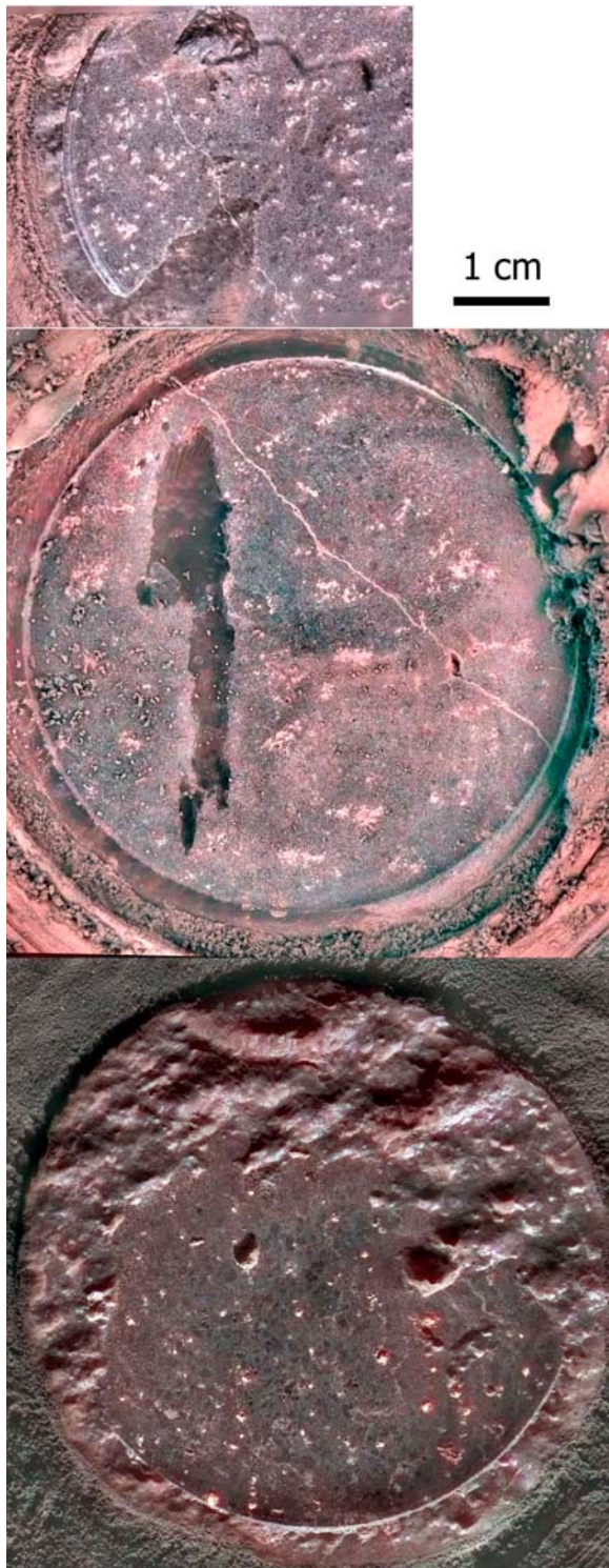
Figure 3. MI images (colorized by Pancam overlays) of RAT holes in rocks; from top to bottom: Adirondack, Mazatzal, Humphrey. Humphrey is illuminated by direct sunlight from the top, whereas images of the other rocks were acquired while they were in shadow.
