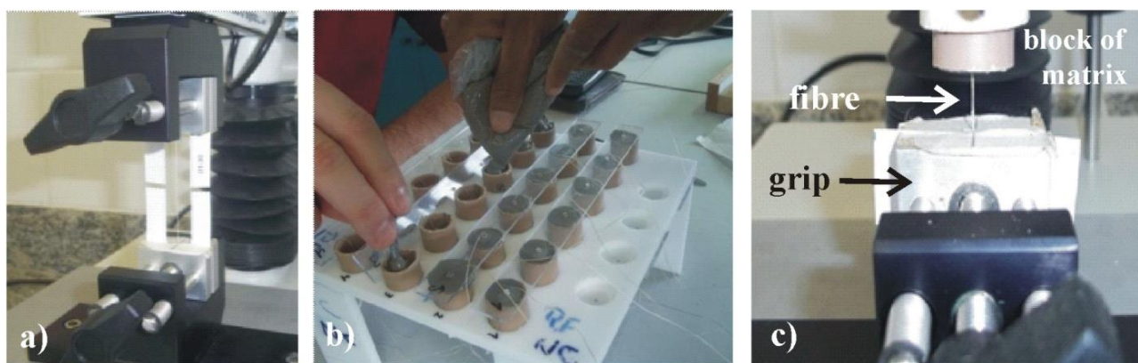
FIGURE 3. Test Methods: a) Tensile test setup; b) Pull-out mold filling; c) Pull-out test setup
