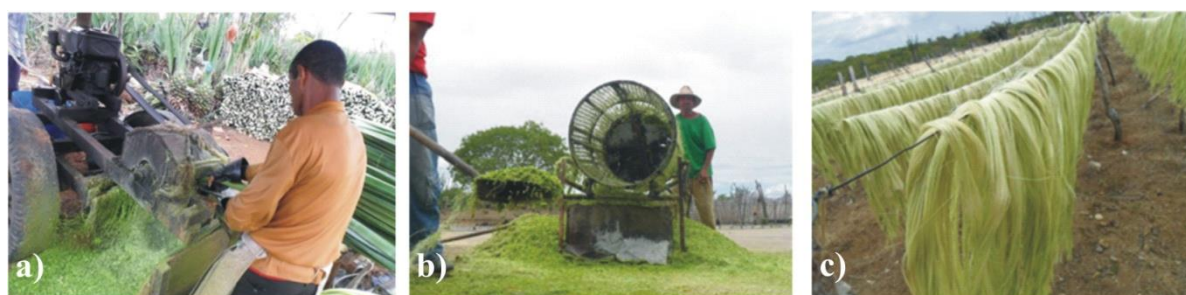
FIGURE 1. Production process of sisal fiber: a) Extraction of sisal fiber; b) Drying of the fiber; c) Separation of the sisal residue
