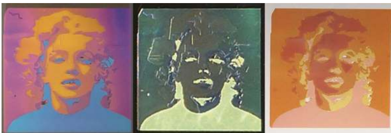
Fig. 2. Color image printed with PICSLUP (1 \times 1 cm), showing the dramatic color change according to the illumination/observation geometry. Left: Specular reflection mode ( 45^\circ:45^\circ geometry); Center: Off-specular reflection mode ( 45^\circ:0^\circ geometry); Right: Transmission mode ( 0^\circ:0^\circ geometry) [1].
