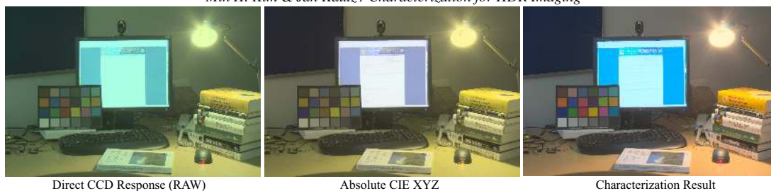
Figure 5: Each step of our characterization method. Direct CCD response RAW is the acquired RAW image without any white balancing. The greenish appearance is due to the infrared filter in front of the CCD, which will be taken care of by the derived mapping. Absolute CIE XYZ is the characterized CIE XYZ image (which we render using a 1:1 mapping to RGB for illustration purposes). Characterization Result is the final image by mapping from characterized and device-independent CIE XYZ to the display sRGB color space.
