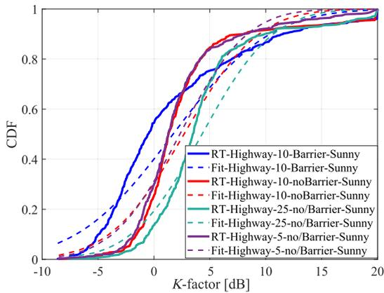
FIGURE 17. Comparison of  $K$ -factor in highway scenario.
