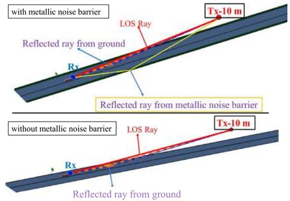
FIGURE 16. Comparison of the same snapshot of the case Highway-10-Barrier and Highway-10-noBarrier.
