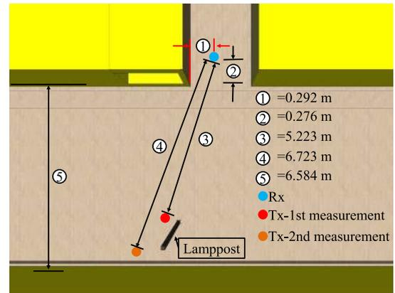
FIGURE 2. Geometry information of the measurement campaign.
