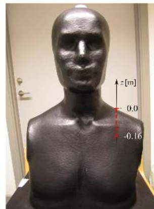
Fig. 8. A human phantom. The dashed line indicates the distance over which the antennas are scanned.
