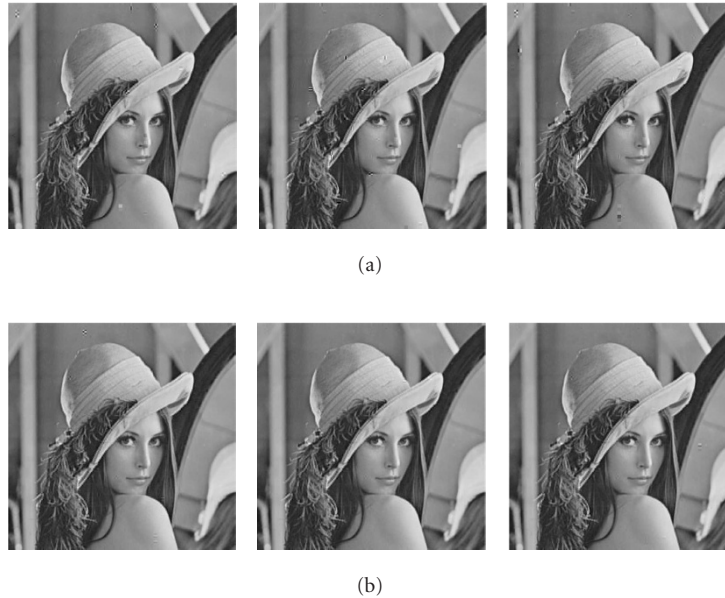
FIGURE 6: Reconstructed image with BER 0.001. (a) Error localization with coding-theoretic approach for DFT frame, DCT frame, and DST frame (from left to right). (b) Error localization with subspace approach for DFT frame, DCT frame, and DST frame (from left to right).
