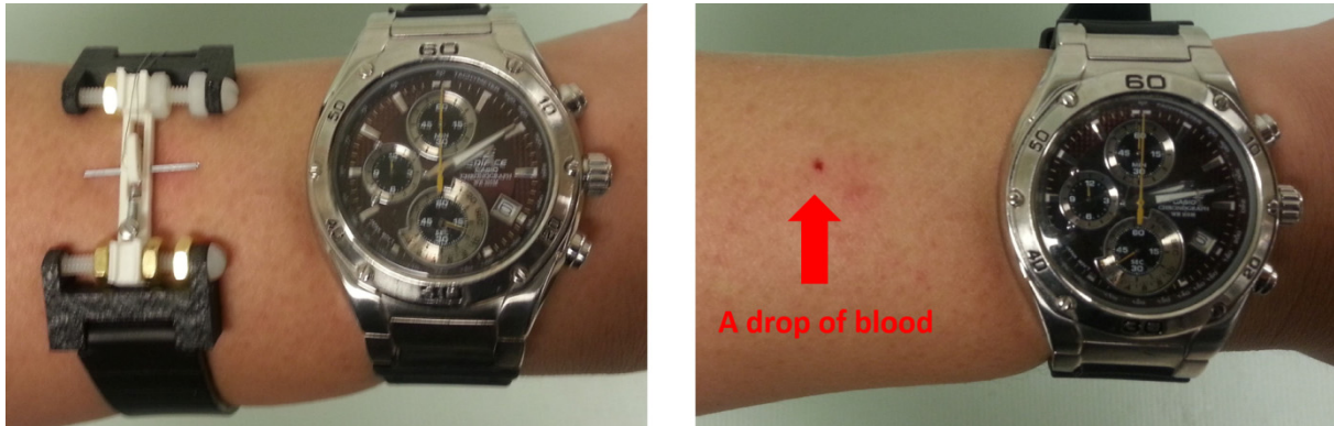
Figure 9. The SMA actuator at the activated state (left); a drop of blood (~1mm in diameter) was observed emerging at the skin surface after the device was removed (right).
