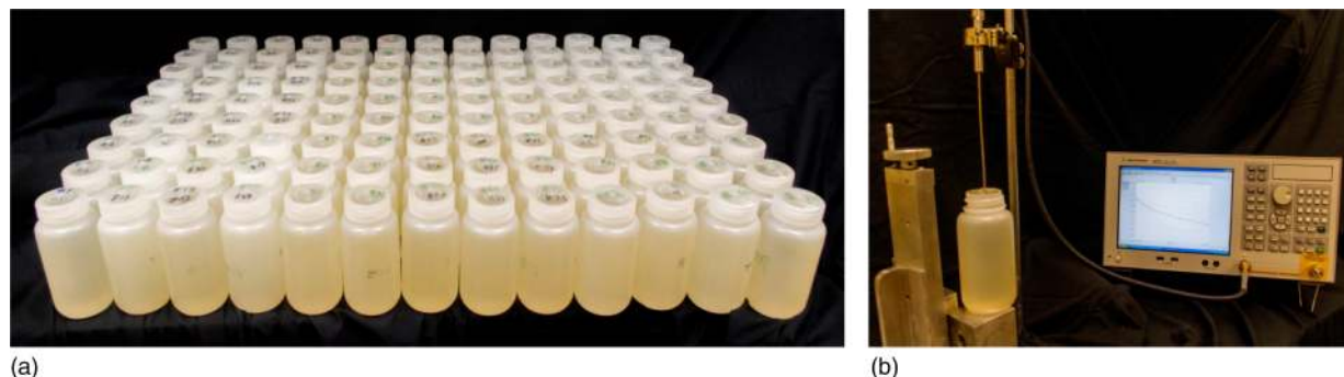
FIG. 1. (a) 9 × 13 phantom sample matrix, (b) experiment setup for dielectric property measurement.
