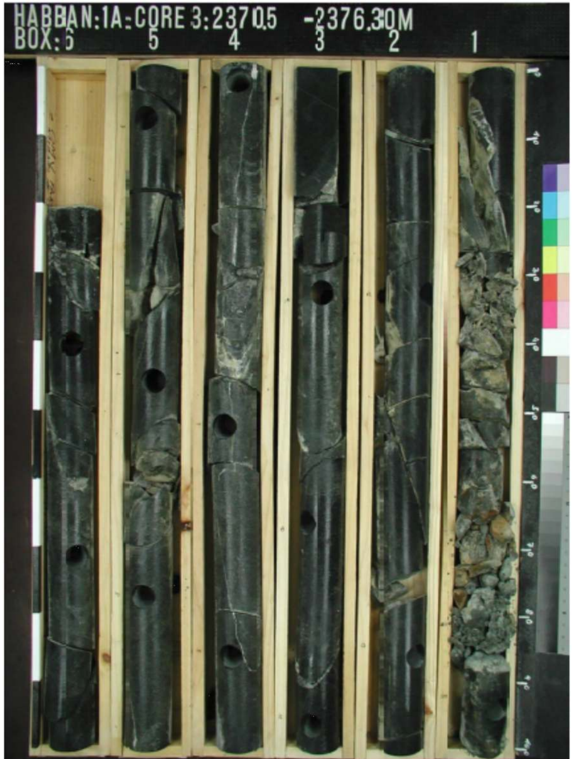
Fig 13. The cored basement reservoir interval 2370.5–2376.3 m at Habban-1 well. Good fracture system is indicated at the samples 1, 4 and 5. Sample 1 is completely crushed.
