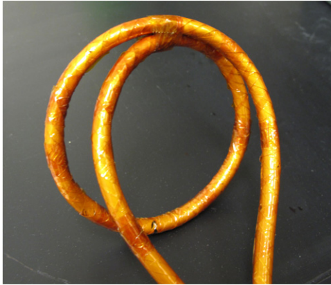
Figure 1. Cable CORC-2 after it was bent into a 12 cm diameter loop.
