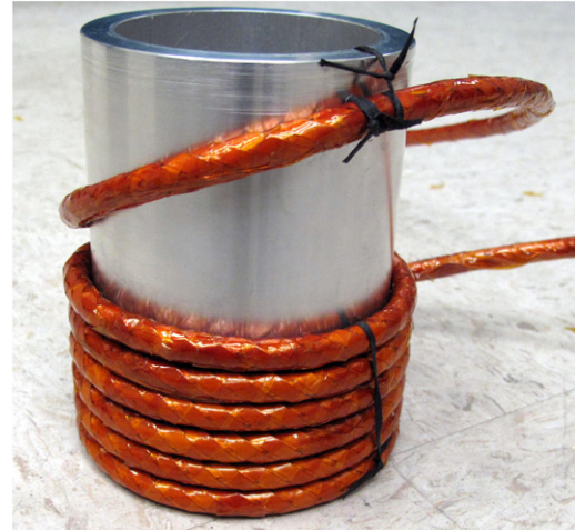
Figure 2. The 6 turns of the inner layer of the magnet that was wound from sample CORC-5.
