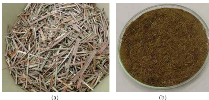
Figure 2. Imperata brasiliensis fibers (a) grounded stems and leaves and (b) sieved fibers after dried.
