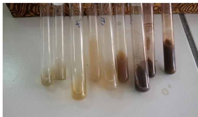
Fig. 1: Solutions of silver nitrate after exposure to the culture supernatant of Bacillus sp. HAI4 (from left to right 0.001, 0.01 and 0.1M ).
