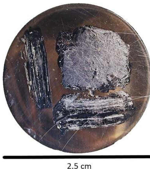
Figure 2. Mica flakes (Sokli10) mounted in epoxy exposing either the surface plane (001) or a cross-section of the crystal
