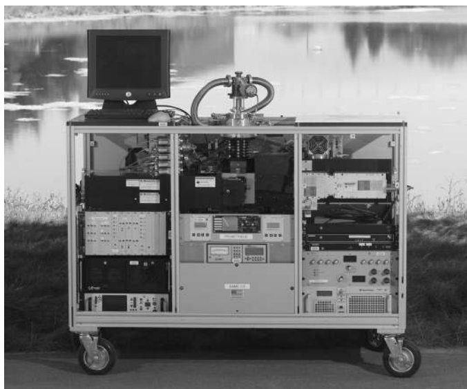
Fig. 1. An image of a BAMS system ready for deployment. The system can easily be transported from location to location and requires only electricity to operate. The virtual impactor is not shown.
