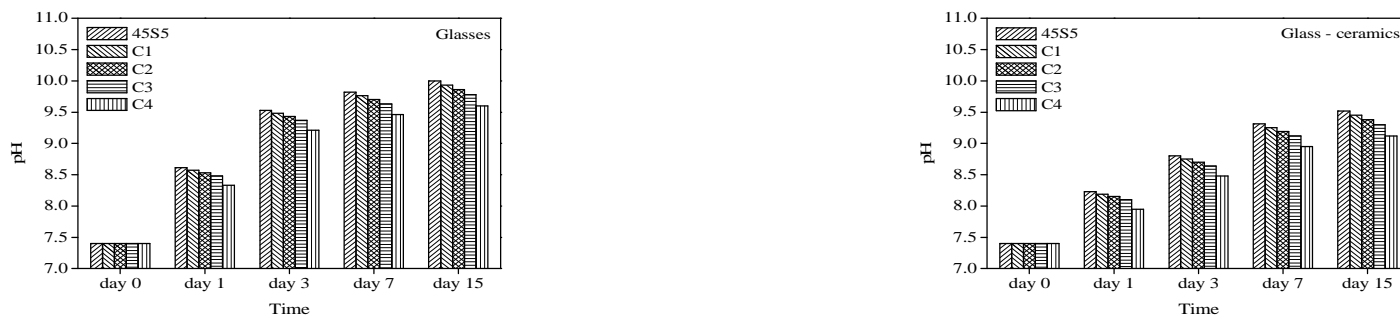
Figure 9: Variation in pH of SBF solution due to soaking for various time periods
