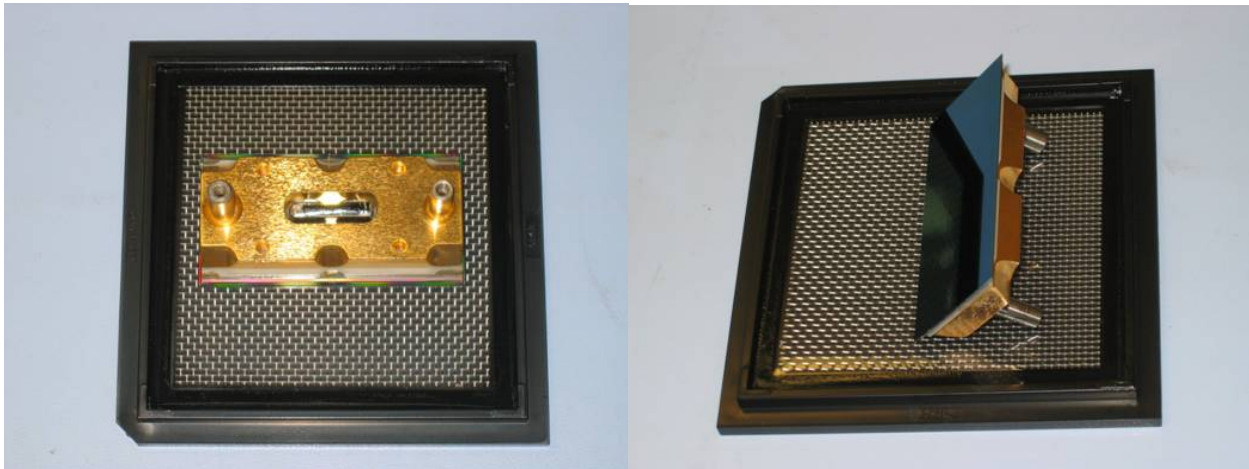
Figure 1-1 A 4-side-butable pedestal package is displayed. View of underside of a pedestal package sitting on a gel-pack showing the Au-plated INVAR foot, two alignment pins, the connector, the edge of the AlN blank with cut-outs for the wirebonds and the edge of the CCD (left). The same CCD viewed in perspective showing the front side of the CCD, which is dark because of the anti-reflective coating (right). The cut-outs in the Au-plated INVAR foot allow the wirebonding machine viewing access to the AlN circuit and CCD bond pads.
