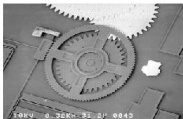
Figure 7. Rotary stepper motor. Main two-level gear adapts thermal actuator stroke to tooth pitch of standard, software-generated Sandia gears. Upper gear is planarized Poly-3.
