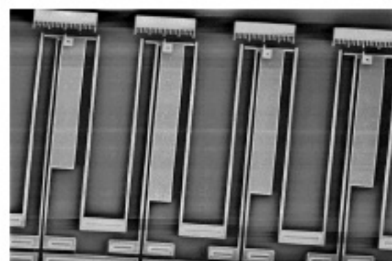
Figure 2. Four independent 150 \mu\text{m} long actuators, each instrumented with deflection scales and two test beams for measuring force in both forward and backward deflection.
