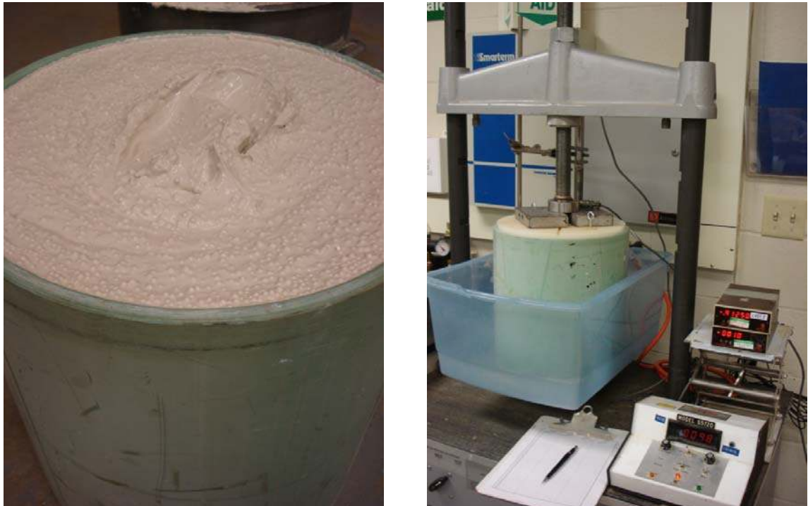
Figure 4.1. Slurry Consolidation (98.5% Kaolin : 1.5% EPS)
