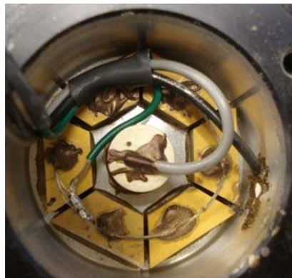
Figure 4.12. Piezoelectric Crystals Mounted in Specimen End Platens
