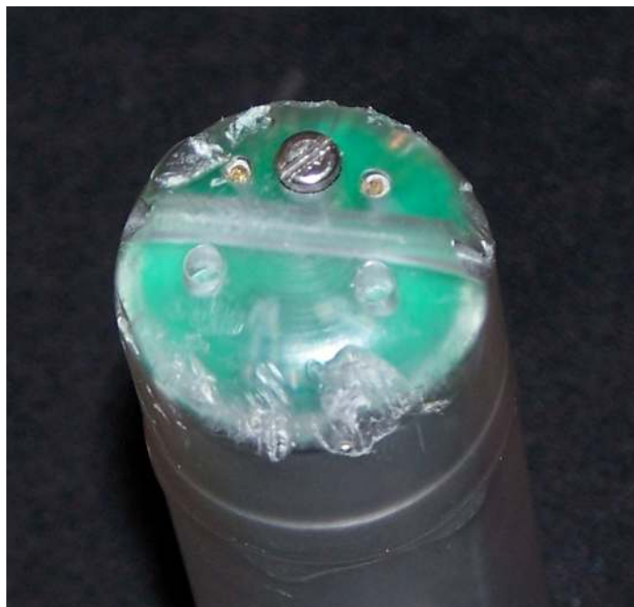
Figure 4.5. Chips and scratches visible on the polycarbonate Sensor Fish casing.
