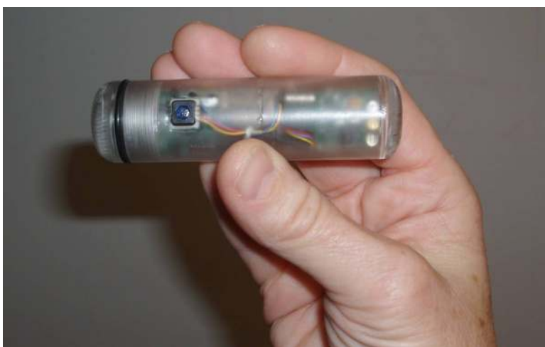
Figure 2.4. Six-degree-of-freedom Sensor Fish device.
